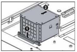
Make sure that the RPS power distribution module is connected to the power supply connector(s) on the power supply(ies).
